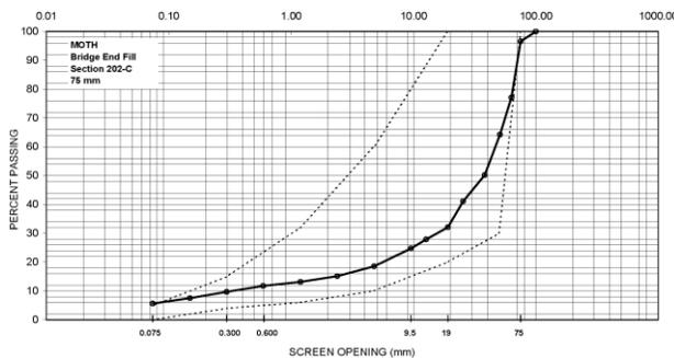
Figure 3. Typical MSE backfill gradation.
