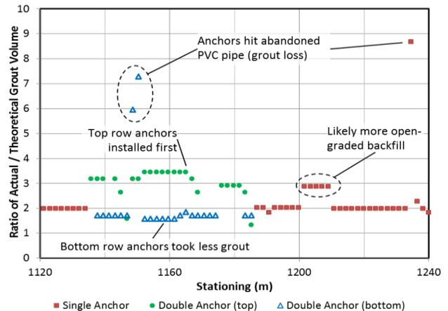
Figure 9. Ratio of actual/theoretical grout volume for the bond length of the anchors.
