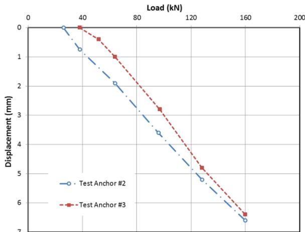
Figure 7. Load-deflection plot for bond stress verification anchors (133 mm diameter hole, 2.5 m bond length).
