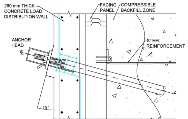
Figure 4. Typical anchor head and concrete blister section.
