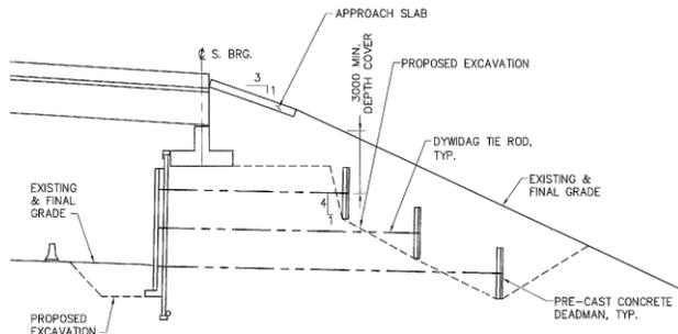
Figure 12. Typical detail of deadman installation for retrofit of a MSE abutment wall at wildlife crossing.
