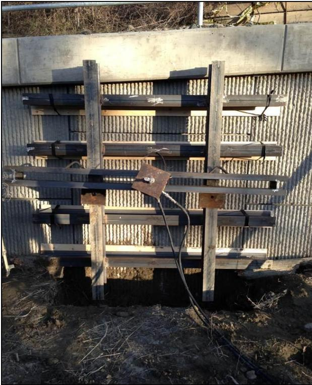
Figure 6. Pull-out test on a sacrificial anchor installed in the MSE backfill zone.
