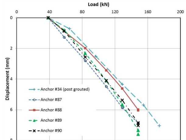
Figure 10. Load-displacement plot for proof tests.
