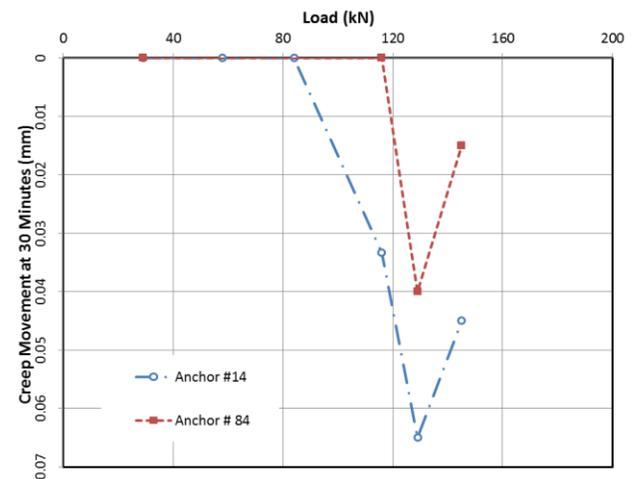
Figure 11. Creep movement versus load measured for two anchors.
